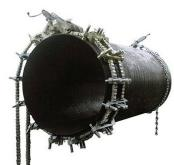
The Mathey Dearman Double Chain Clamp is a heavy-duty vessel clamp designed for alignment and reforming of pipes and vessels up to 20' (6 m) in diameter with Schedule 80 wall thickness.
