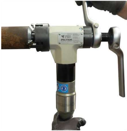
US25CH with pneumatic drive
