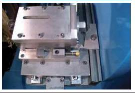
The main feature of the Protem US600-R is its copying carriage, which allows the US600-R to perform any type of weld preparation such as, I-bevel, J-bevel, V-bevel, compound bevel, etc. with accuracy and repeatability. The US600-R can also machine any type of material, for instance; carbon steel, stainless steel, alloy, inconel, duplex or super-duplex. Our R&D engineers are able to adapt the machine to any type of welding preparation and material upon request.
