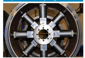
The Protem US600-R is stabilized with a spider clamping kit which was designed to adjust the concentricity and squareness between the tube and the machine. This system is extremely accurate even with large diameter tubes.
