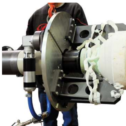
PROTEM US with coating removal option
