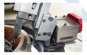
The counterboring carriage performs an ID bevel in order to obtain a regular land.
