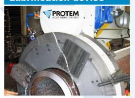
In order to increase the lifetime of the inserts and to reduce the noise level during the machining operations a lubrication device must be used. This lubrication device is made up of a cutting fluid tank, covered by a chip container and a pump for circulating the cutting fluid . A flexible piping kit for aiming the fluid at the cutting point is also supplied together with a tank support plate. This option is activated through a push button.
