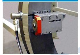
100 mm (3.937") stroke carriages or two ovality tracking carriages are necessary. Depending on the application, a wide range of cutting or beveling tool bits are available to perform the majority of the required machining applications.
