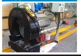
The whole range of TNO units is fitted with a protective housing which covers the tool-plate. The housing represents a safety system for the operators. It has a slot to be able to adjust the posit ion of the clutch pin that moves the tool carriage forward.
