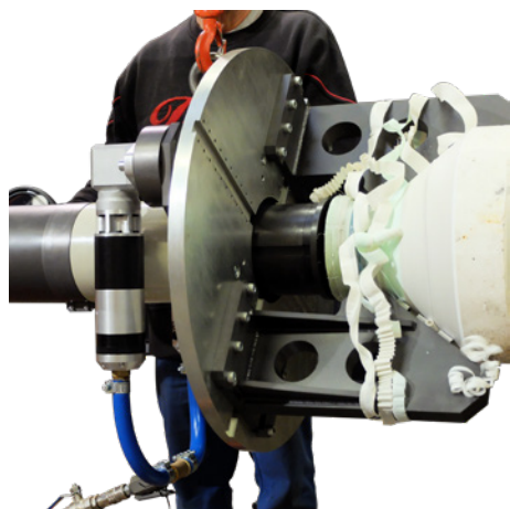
PROTEM US with coating removal option
