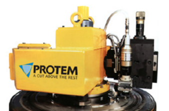
US 480 R – Machining and Cladding Equipment on Steam Generator
