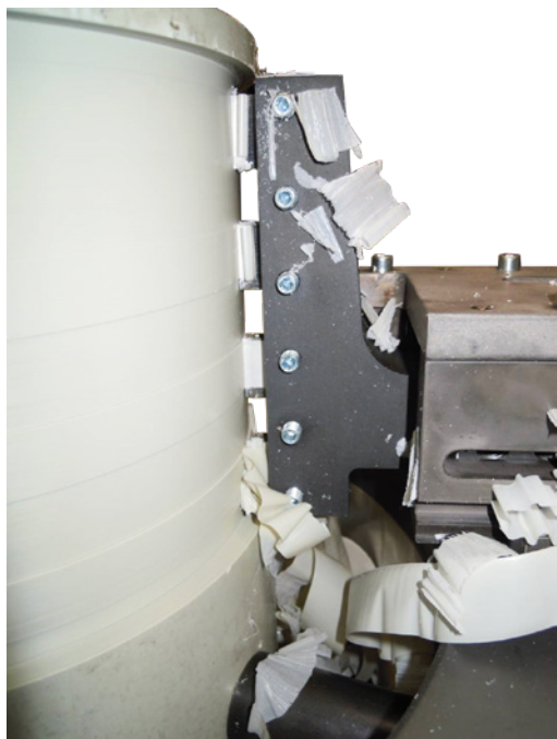
PROTEM TTNG Orbital cutting machine with coating removal option
