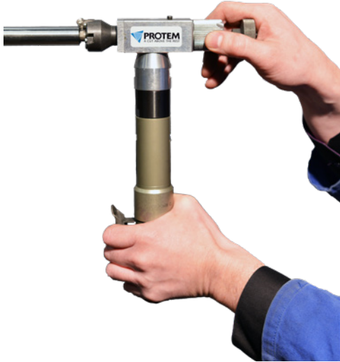
SM8 with pneumatic drive
