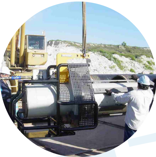
Rollers located at the top of the clamping mandrel to ease its access to the tubes.
