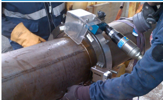
TTLW323 Tube Cutting & Beveling Equipment with pneumatic drive
