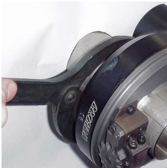
Operation 3: Clamping of the machine nut on the tube.
