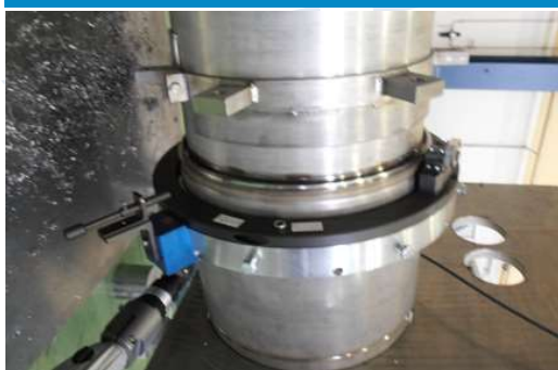
TTLW508 Tube Cutting & Beveling Equipment with pneumatic drive
