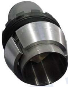
Operation 2: Implementation and assembly of the two half-shells on the tube.
