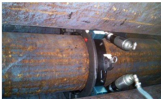
TTLW168 Orbital Tube Cutting & Beveling Equipment with pneumatic drive
