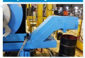
The optional chips conveyor can be used on all versions of the CTA. This option increases productivity as all the chips produced during a machining cycle are removed automatically.
