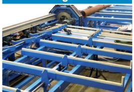
All the feeding tube conveyors or storage tube conveyors can be easily connected to any machine in the CTA series.
