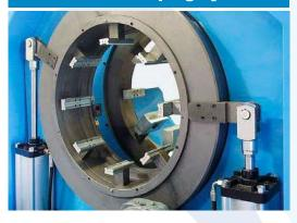
The automatic and pneumatic clamping systems set the concentricity of the tube. The machining is performed between both clamping systems.
