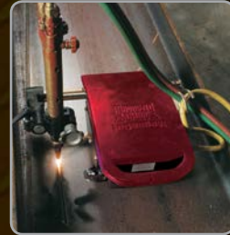
Vertical or horizontal I-beam 20" (508mm) wide or wider can be precision cut with the MagnaCut XM
