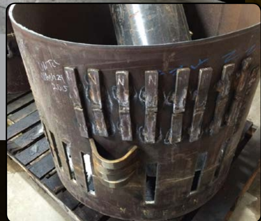
An excellent tool for making coupons for bend, tensile strength, and hardness tes
