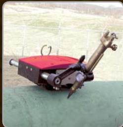
Pipe diameters 16" (406 mm) and larger can be cut lengthwise.
