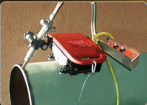
MagnaCut XM can be used on pipe with coating up to 0.015" (0.4 mm) thick.
