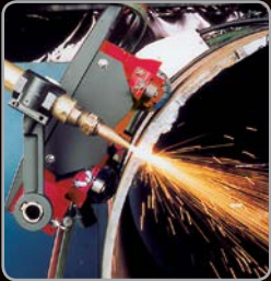
The MagnaCut XM cuts outside diameters 6 5/8" (167 mm) and larger.
