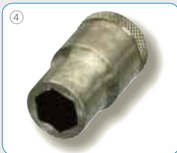
Outside diameter turned and knurled. For this and the next step, GEDORE uses high-tech machinery from its in-house special mechanical engineering department.
