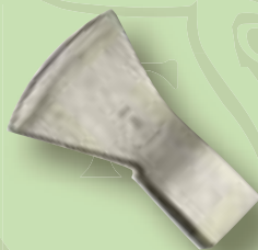
⑥ Sand-blasting the surface. Fine-grinding the cutting edge. A crowned cut increases stability. Transparent varnish protects the axe head from corrosion.
