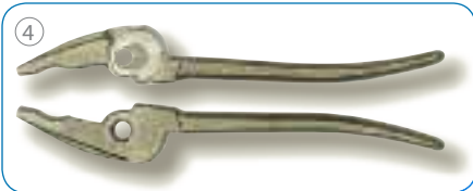
The head is machined in a CNC-controlled machining centre. The rivet hole is drilled and counter-bored. The joint clearance and the outer contour are milled. The geometry of the joint area and the coarse and fine toothing are broached.
