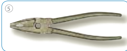
The joint faces are precision milled. The pliers head takes on its final form.
