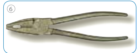
The moving and fixed pliers legs are riveted together. A smooth-moving joint with no play is the essential requirement for safe one-handed operation.
