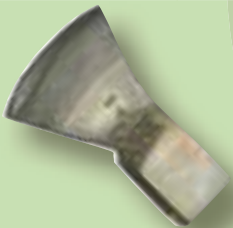
⑤ Permanent marking by means of a stamp bearing the manufacturer's symbol. Tempering (hardening and tempering) the cutting edge ensures hardness and toughness.
