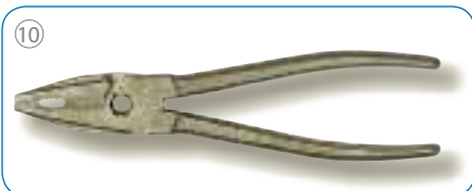
The surface is cleaned by sand blasting. The removal of scale and grease is necessary for the follow-on electroplating process.
