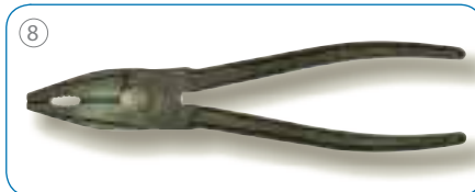
The cutting edges of GEDORE pliers are once again induction hardened. The additional hardness that this achieves ensures a good cutting performance and a long life between sharpening.
