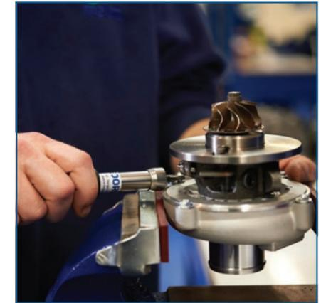
**Improved accuracy, consistency and control.** Accurate process control is ensured by reducing the risk of under and over tightening, due to unique Breaking Technology. This gives the operator more time to react once the target torque is reached
