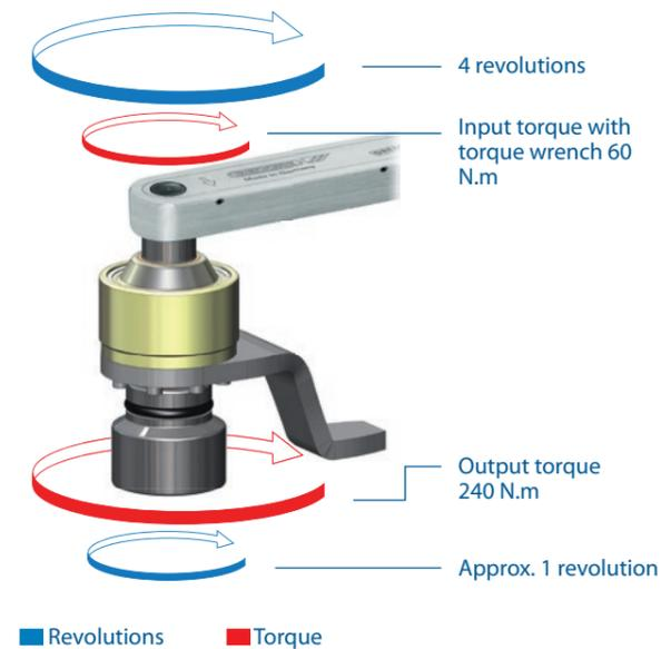
The diagram representation demonstrates the principle of torque multiplication. Let us assume a 60 N.m input torque and a 240 N.m output torque. At a 1:4 ratio, 4 revolutions are needed at the 60 N.m input for 1 revolution with a 240 N.m torque to be obtained at the output.
