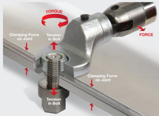
Torque is the application of a **Force** acting at a radial **Distance** and tending to cause rotation. Torque is used to create tension in threaded fasteners
